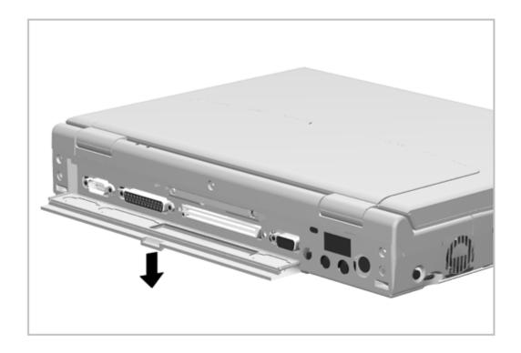
Figure 5-17. Removing the Connector Cover
